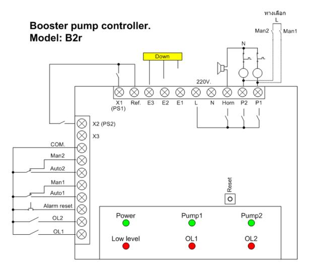
Dimension: 164x164x45 mm3. Level electrode: 3 Alarm clause: low level and motor overload. Delay off timer: 0, 5,10,15 sec. Power supply: 220V.
