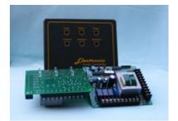
Booster pump controller with LED.
